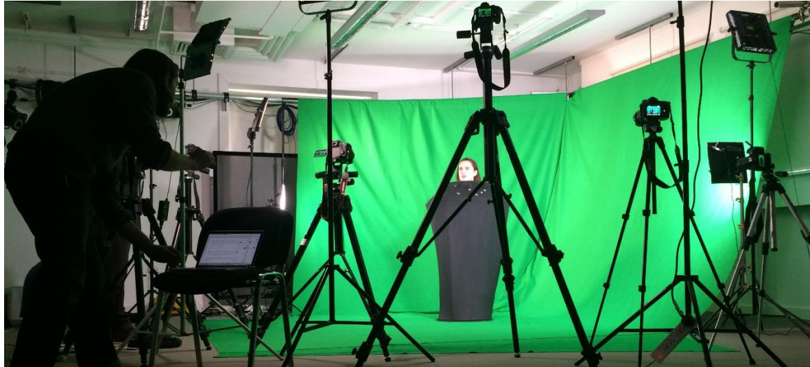
Fig. 2: Camera setup in 150-degree arc, with director and actor on set. © V-SENSE
