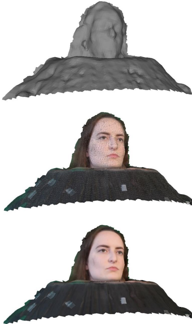
Fig. 3: (from top to bottom): a) reconstructed 3D mesh, before texturing; b) textured model with mesh wireframe; and c) final photorealistic model. © V-SENSE
