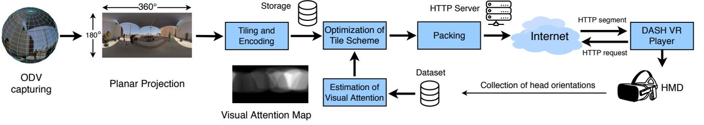
Fig. 1: Schematic diagram of the proposed adaptive ODV streaming system for VR.
