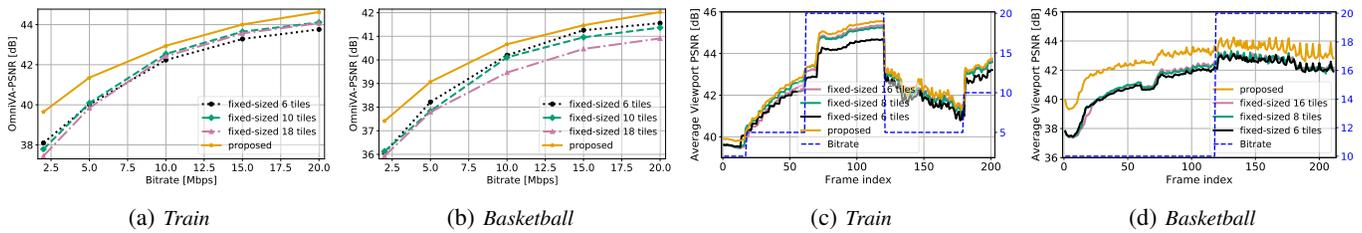
Fig. 4: (a,b) Performance comparison using the RD curves computed with the average OmniVA-PSNR. (c,d) viewport-PSNR quality over frame between the proposed and the reference methods on varying bandwidth (Mbps).
