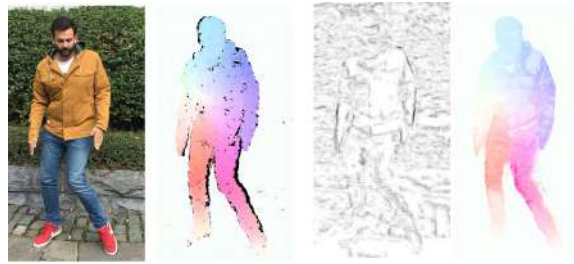
Figure 3: Pictured left to right, the STEA flow processing pipeline: input RGB image from a given viewpoint, (1) CPM nearest neighbour field estimate, (2) SED detected edges, (3) interpolated dense STEA output. Conventional colour coding has been used to illustrate the orientation and intensity of the optical flow vectors. Orientation is indicated by means of hue while vector magnitude is proportional to the saturation i.e. negligible motion is represented by white, high-speed motion is shown in highly saturated color.
