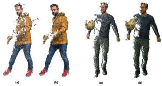
Figure 5: Filtered point clouds from two sequences, one extracted from hand held cameras in outdoor setting (left) and the other captured in a green screen studio (right). Both show a comparison between the point cloud extracted from framewise reconstruction (a), and the filtered results (b).
