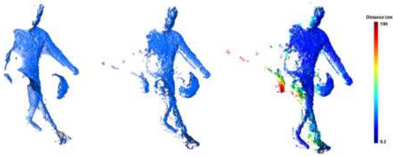
Figure 4: A visual representation of the coherent merge process. Pictured is the result of merging the predicted point cloud (left) with the target cloud (middle). All points are color-coded with respect to the distance between their nearest-neighbour match in the other cloud. Points labelled higher than the threshold for the given frame will be removed from the merged result.
