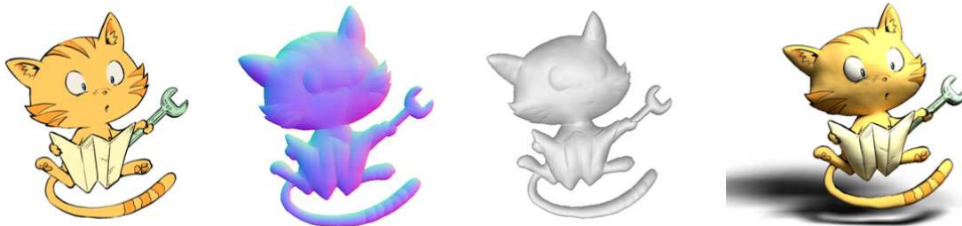
(c) From left to right: input drawing, predicted normal map, inflated mesh, global illumination example
